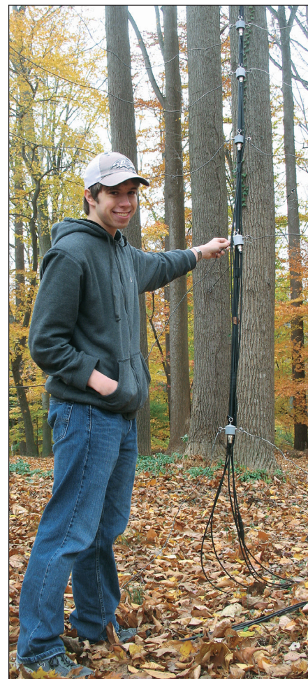
Figure 2 — The five SO239 dipole connectors attach the loops to 75 \Omega coax quarter wave matching sections. Brad, KB3MNE, points to the 17 meter connector.
